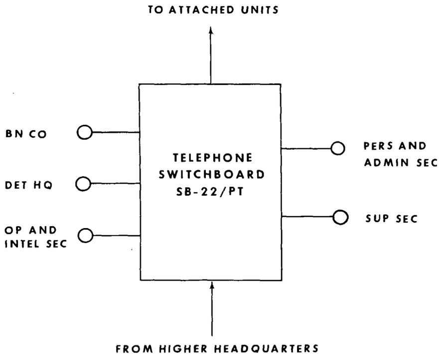
Figure 22. (Superseded) Type wire system of a chemical service battalion headquarters and headquarters detachment.
