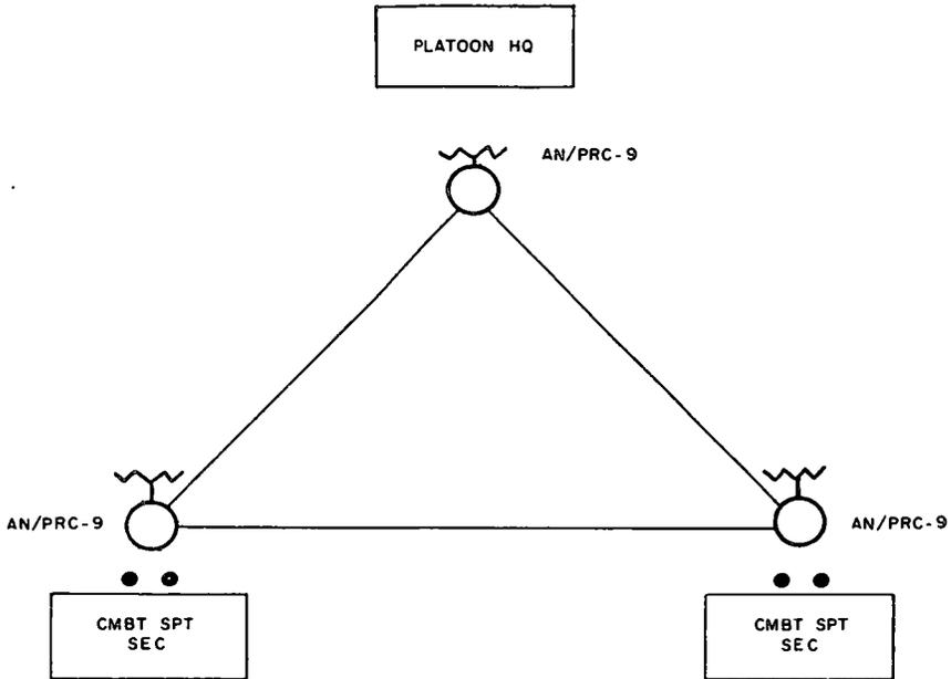
Note: The two radios shown with the Combat Support Sections can be used instead to provide communication for two Radiological Survey Parties, CBR Reconnaissance Teams, Smoke Generator Sections, or other work parties.
