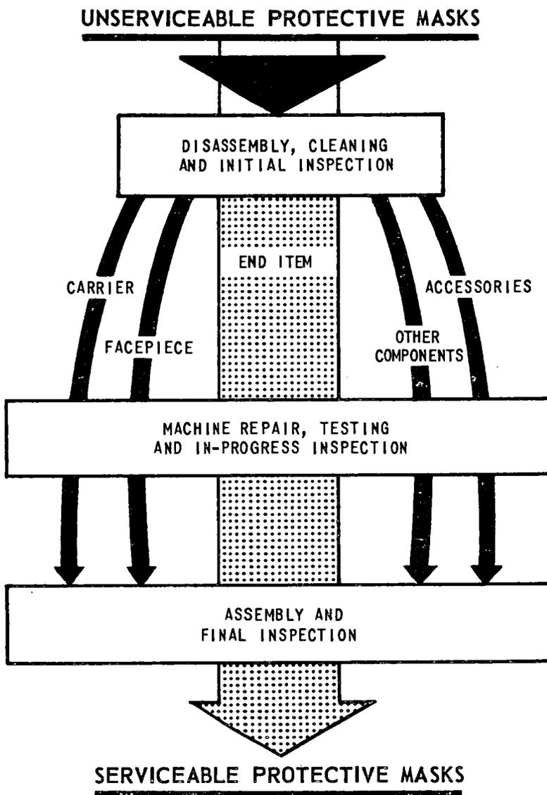
Figure 5. Production line maintenance of protective masks.
