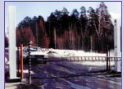
Vehicle Portal Monitor at Chelyabinsk-70
