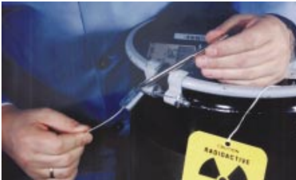
Figure 6. Tamper-indicating device on nuclear material container
